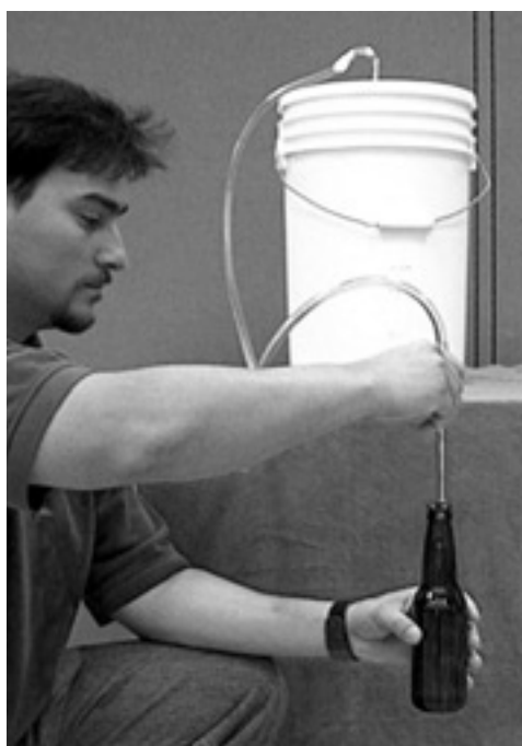
Figure 14 —Filling bottles from a siphon with a bottle filler attachment.
